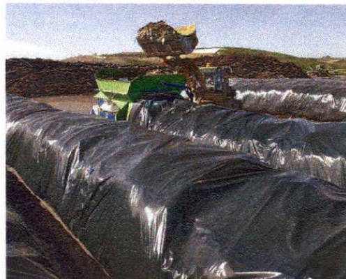
4 th - This material is bagged like sausage, "cooked" for 3 months, and then large items are screened out.
